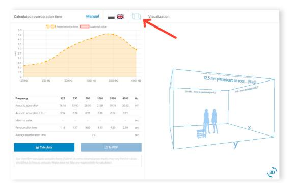
12. Visualization of the room – you can open an additional window with 3D visualization of the room by clicking the button in top right corner, marked with "cube". There will be visible doors and windows on selected walls, some furnishing elements will be visible as well. Block can be turned around and seen from every side. Next clicking in "cube" button will close the window with a view of the room.
