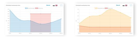
**9.** After correct input of data for all surfaces the second line will appear on the chart – calculated reverberation time or acoustic absorption, and the figures with results will appear in the table. Additionally the proper statement about fulfilling or not the requirements of a standard PN-B-02151-4 will appear as well.
